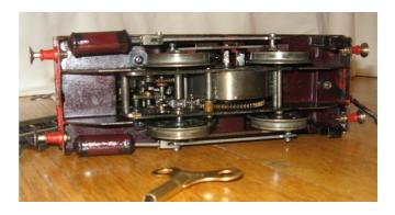
The mechanism is truly beautiful. An enormous spring which takes some winding, a complex gear train and a mechanical regulator (basically a brake) which keeps the speed down even when the spring is fully wound. Two rods at the back control a reversing gear and a lock which holds the engine stationary.
